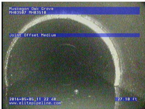
GM3676_29b5a4f6-782c-44a4-b604-e6dda5d2d56c_20160505_112417_126.jpg, 00:04:44, 27.09 Joint Offset Medium
