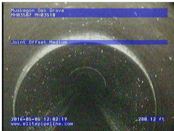
GM3676_29b5a4f6-782c-44a4-b604-e6dda5d2d56c_20160505_120356_056.jpg, 00:35:29, 280.12 Joint Offset Medium
