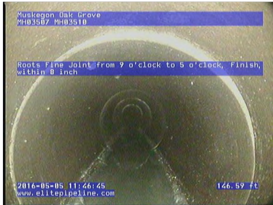
GM3676_29b5a4f6-782c-44a4-b604-e6dda5d2d56c_20160505_114822_035.jpg, 00:22:11, 146.58 Roots Fine Joint from 9 o'clock to 5 o'clock, Finish, within 8 inch
